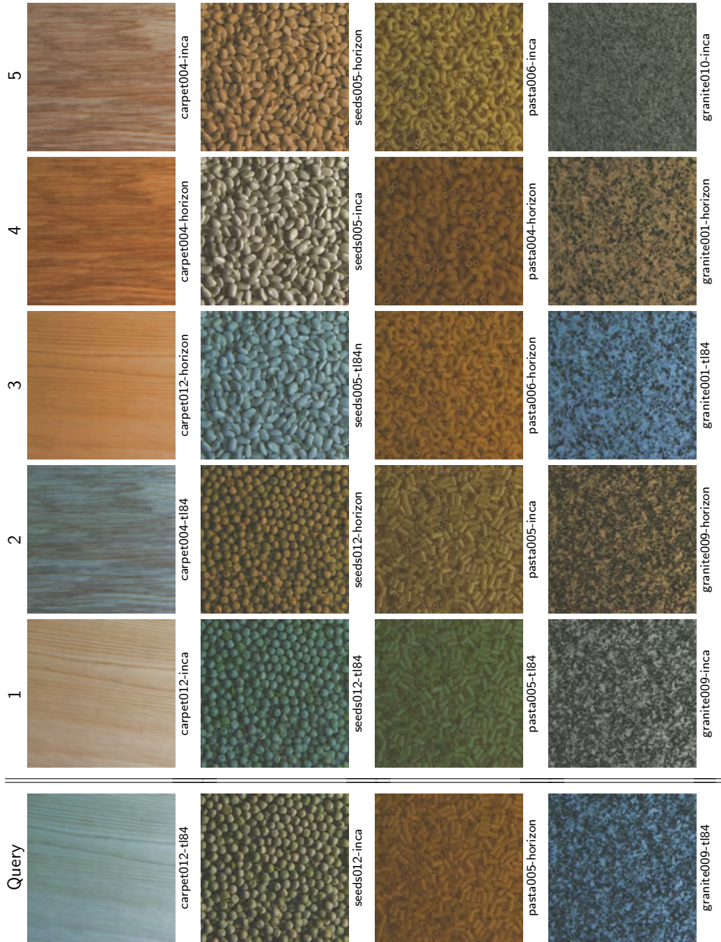
Figure 4: Examples of illumination invariant retrieval from Outex texture database [28], which contains materials illuminated with tree different illumination spectra (inca, horizon, tl84). The query images are followed by retrieved images in order of similarity. The images of query materials acquired under different illumination spectra were successfully retrieved at positions 1 – 3.
